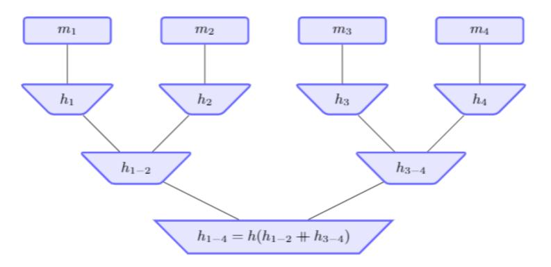
$$\mathcal{MT}.\Delta(M) \equiv \begin{cases} \text{If } L = 0: \quad h(m_1) \\ \text{Else} \quad \quad h(\mathcal{MT}.\Delta(m_1, \dots, m_{2^{L-1}}) \# \\ & & & \mathcal{MT}.\Delta(m_{2^{L-1}+1}, \dots, m_{2^L})) \end{cases}$$
